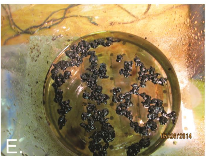
Figure 3. Osprey Spill Control Cellulose Sorbent - Diesel on Water Test. A. on diesel, B. after 10 sec., C. during test, D. 2 min post-test, and E. 2 min post-test viewed from the top of the test jar.
